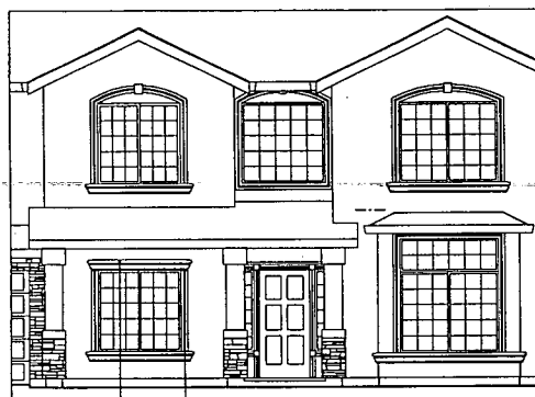
① (BAY 1) ② (BAY 2) SIMILAR AT OTHER ELEVATIONS. TRIM SURROUND AT WINDOWS TO MATCH THE TRIM AT LIVING ROOM WINDOW ① ELEVATION "A" 1/4" = 1'-0" SEE SHEET 1 FOR GENERAL NOTES
