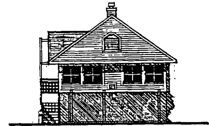
NORTH ELEVATION - NEW CONSTRUCTION
