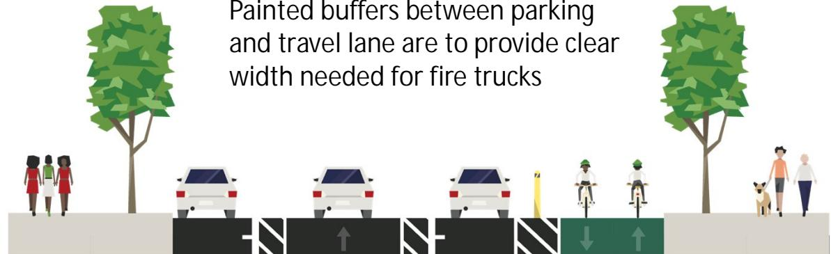
Painted buffers between parking and travel lane are to provide clear width needed for fire trucks
