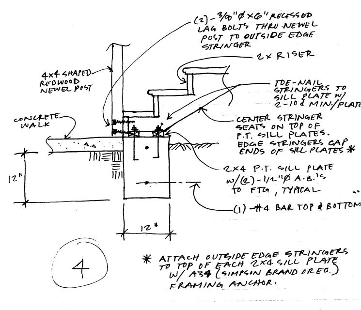
COTAIR END FRAMING DETAIL NO SCALE
