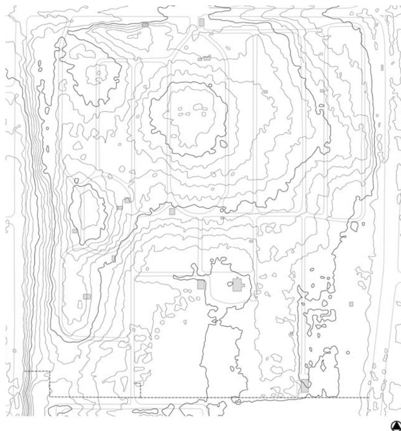
Figure 2.1 Topography Map Scale: 1" = 300' Contour Interval = 2'-0"
